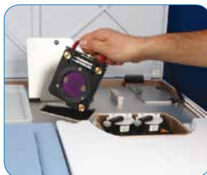
Beamsplitters are easy to exchange and can be stored inside the optics bench.
